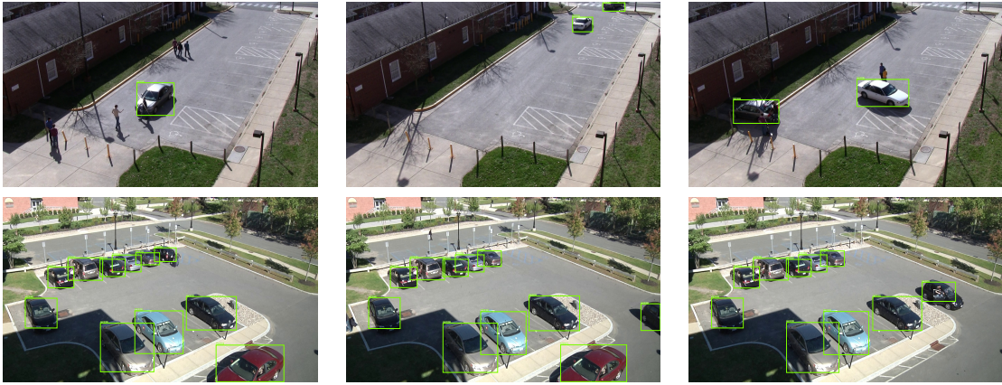
Figure 4.8: Object detection performance of Faster-RCNN trained on 100k images generated by ADR
