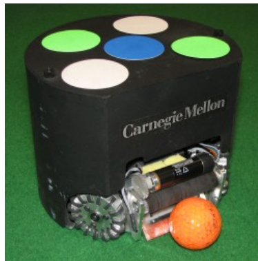
Figure 2.2: One of CMDragon’s robots, with a ball touching its dribbler bar (horizontal black cylinder). The dribbling bar can be spun to put backspin on the ball for semi-control. Designed and built by Michael Licitra.
