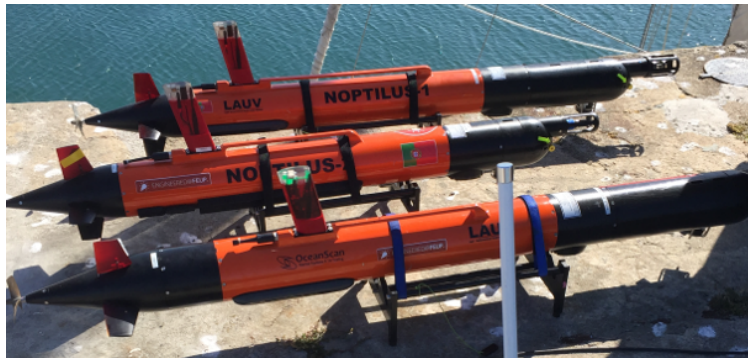
Figure 6.1: Three Light Autonomous Underwater Vehicles (LAUVs) from the Laboratório de Sistemas e Tecnologia Subaquática (LSTS) in Porto, Portugal that were used to gather the depth data in Figure 6.4.
