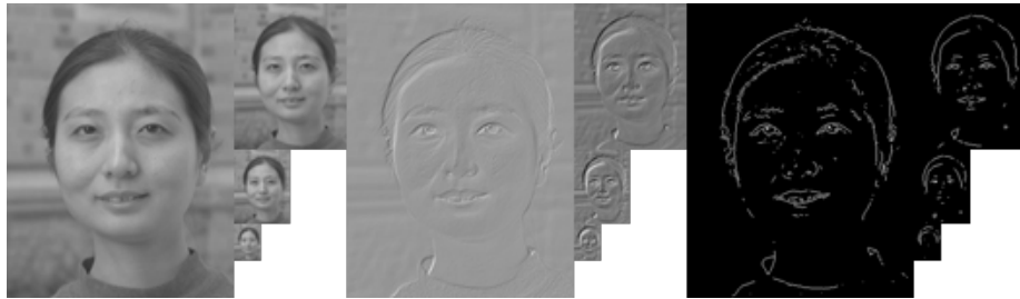
Figure 5: Image, Gradient, and Sobel Edge Intensity pyramids used for multi-resolution search. Individual profile models are extracted to represent the neighborhood surrounding each landmark point at each level of the pyramid.
