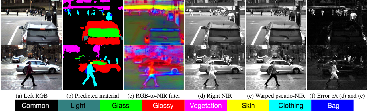
Figure 3. Intermediate results. (b) is the material recognition result from DeepLab [3] (explained in Section 4.2). (c) shows the RGB-to-NIR filters corrected by exposure and white balancing. The R,G,B values represent the weights of R,G,B channels. Some clothing fails in spectral translation because the relationship between its RGB and NIR intensities is low. The structural similarity term in alignment loss (Equation 3) can partially solve this problem as long as the structure is preserved.
