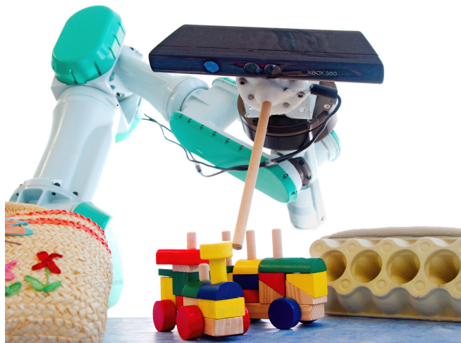
Fig. 1: Our robot arm autonomously interacts with its environment to segment a scene into objects.
