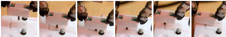
Fig. 10: Sensorimotor primitive sequence for the curved groove peg-in-hole task.
