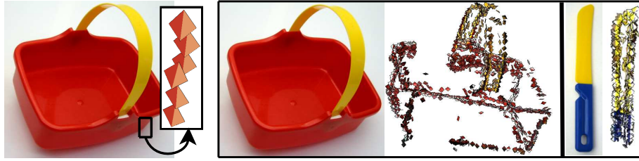
Figure 12: ECV descriptors. Left: ECV descriptors are oriented appearance patches extracted along contours. Right: object-segmented and refined ECV descriptors via structure from motion.
