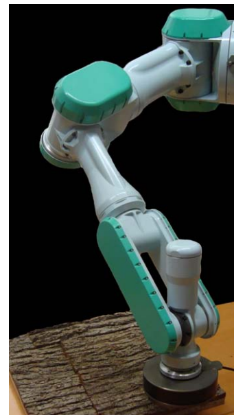
Figure 6.1: Robot learning about materials by stroking and visually inspecting different surfaces
