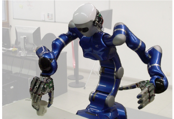
Fig. 1. The Justin robot learns to grasp and lift-up a mug by imitation. The reach-and-grasp movement is learned from human demonstrations. Latent-space dynamic motor primitives generalize the learned movement to new situations.
