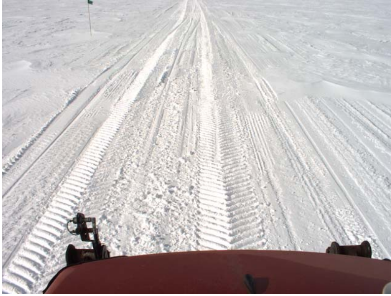
[Scene showing densely packed snow, note the lack of sinkage in the ruts.]
