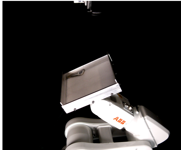
Figure 7. Experimental setup. An industrial robot tilts an allen key, with April Tag attached, in an aluminum tray. The overhead camera records the pose of the allen key after each tilt.
