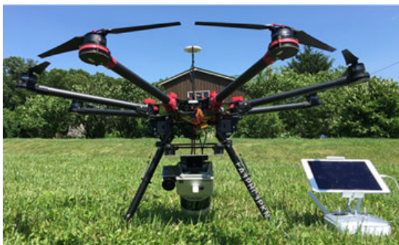
FIGURE 32 Drone platform used in air-ground collaborative mapping test. This is a DJI S1000 aircraft mounted with a sensor suite which has the same sensor setup as in Figure 16b [Color figure can be viewed at wileyonlinelibrary.com ]
