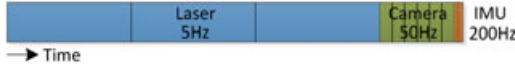
FIGURE 12 Illustration of transform integration. The final motion estimation is integration of the 5-Hz scan matching output (blue), the 50-Hz visual-inertial odometry output (green), and the 200-Hz IMU prediction (orange), at the IMU frequency. The density of the vertical line segments in each section indicates the motion estimation frequency from the corresponding module. IMU: inertial measurement unit [Color figure can be viewed at wileyonlinelibrary.com]
