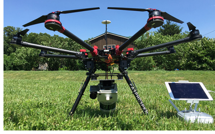
Fig. 9 DJI S1000 aircraft with sensor pack. The aircraft is built with a GPS receiver (on top of the aircraft). GPS data is not used in mapping or autonomous missions as in this paper.
