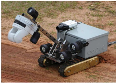
Figure 1.2: A tethered crawler designed at Savannah River National Labs for inspection of the H-canyon exhaust tunnel in 2009 [28]. This vehicle is part of a series of remote-controlled vehicles built specifically to determine the conditions inside the tunnel and check for structural concerns.
