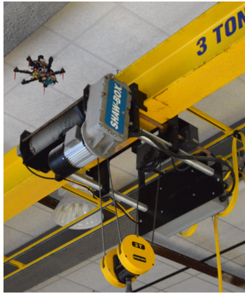
Figure 1.3: A hexrotor flying above an indoor crane to use its downward facing sensors to inspect the gantry and crane below.
