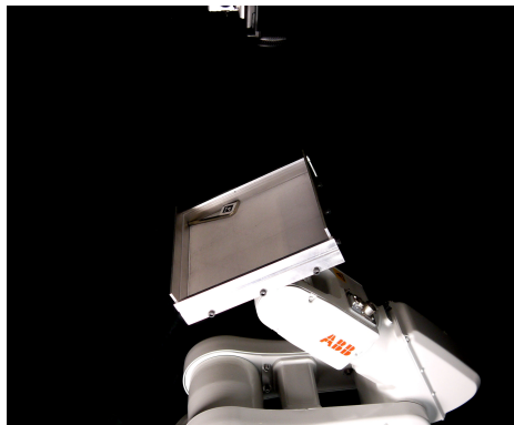
Fig. 7: Experimental setup. An industrial robot tilts an allen key, with April Tag attached, in an aluminum tray. The overhead camera records the pose of the allen key after each tilt.
