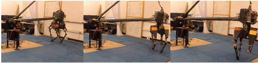
FIGURE 5.3: A time lapse of ATRIAS walking around the boom during a run of DoG-based kernel.
