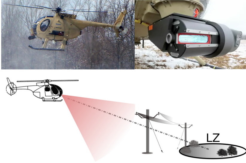
Figure 4.1: Application Scenario: Top Left – Test Vehicle, Boeing Unmanned Littlebird. Top Right – Near Earth Autonomy M3 sensor suite, equipped with a actively controllable high range laser. Bottom – Example mission scenario, the vehicle is suppose to autonomously navigate to a pre-defined landing zone at high speeds, evaluate it and decide to whether to land or not while ensuring safety.
