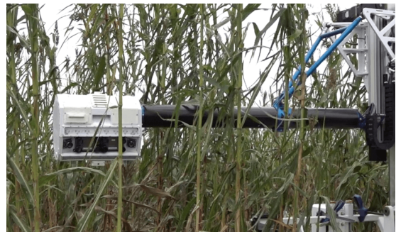
Fig. 2. A closeup of the multi-camera sensor pod deployed on the robotic platform. The sensor pod contains eight forward facing and two additional cameras verged on either ends at an angle of 30°. The sensor pod is connected to a robotic arm and can collect images at multiple plant heights.
