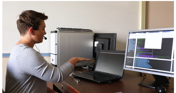
Figure 1: User study setup for the multimodal interface. The user speaks into the headset while performing gestures over the Leap Motion controller.
