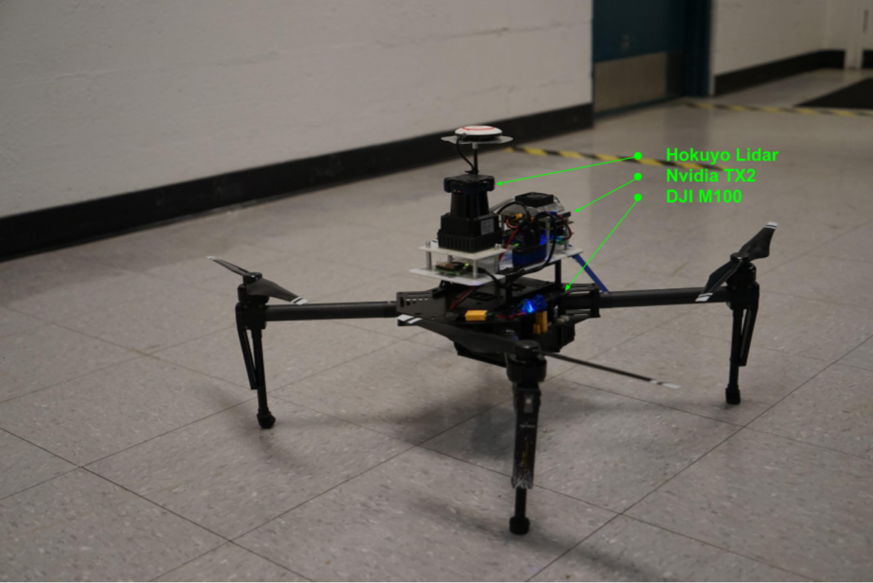
Figure 4.8: Robot equipped with 2D Lidar and Nvidia TX2
