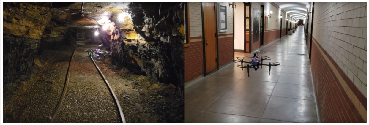
Figure 4.7: Left: Quadcopter flying with learned policy in a coal mine. Right: Quadcopter flying with learned policy in hallway environment.
