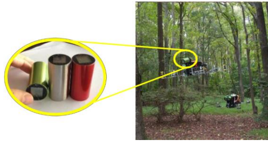
Fig. 1. Example ozone sensor used on a UAV for collecting atmospheric data [10].
