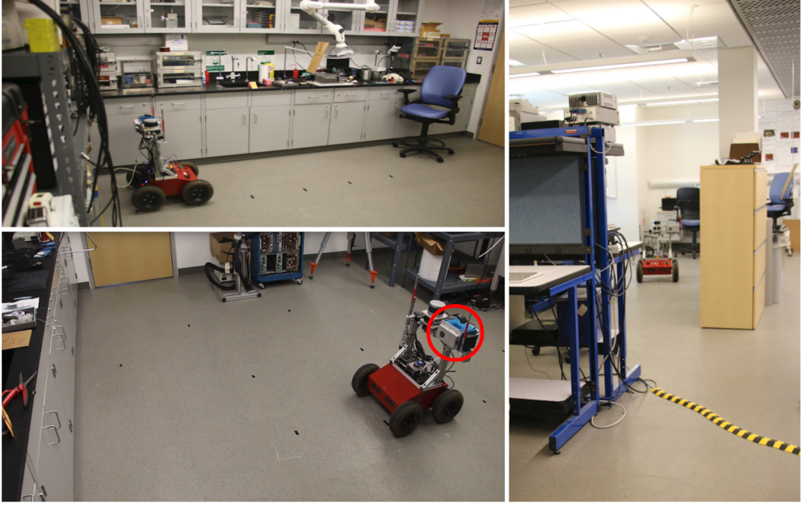
Figure 2.5: Collage of experiments being carried out in the small (top left and bottom left) and large (right) laboratory environments with a ground robot equipped with a gamma camera (circled in red).
