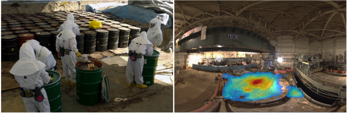
Figure 1.1: Left: Retrieval of nuclear waste stored underground at the Hanford Site in the 1970s and 1980s [5]. Right: Imaging of a radiation hotspot at a reactor in Fukushima using a gamma-ray camera [6].
