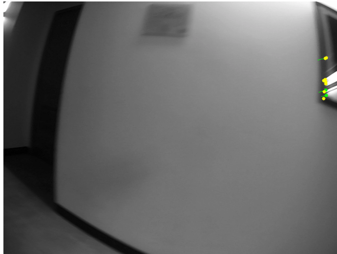
Figure 4.13: Image capturing the point of failure of visual-odometry system. Sparse texture coupled with motion blur produce insufficient contrast for feature extraction.
