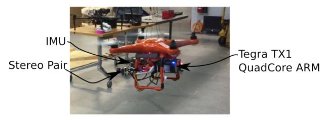
Figure 4.11: Robot-2: A smaller quadrotor platform used for experiments: equipped with stereo camera sensor suite and onboard ARM computer
