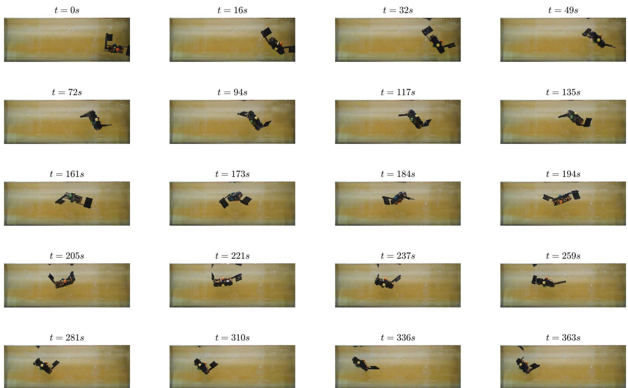
Figure 3.13: Snapshots of the side view of the 3D Swimmer executing the translation gait
