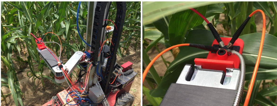
Figure 5.1: The leaf grasping manipulator during initial field testing
