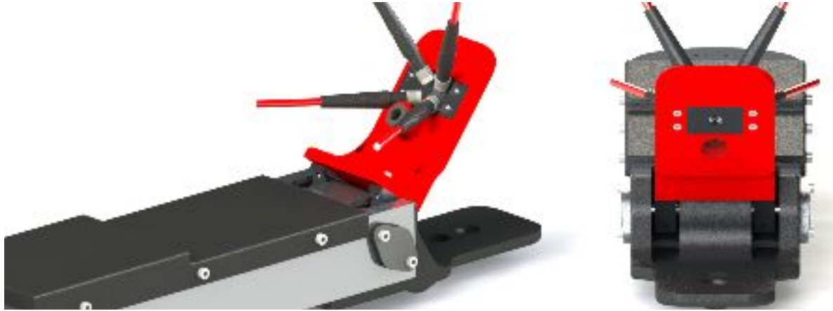
Figure 3.4: Custom leaf clamp end effector
