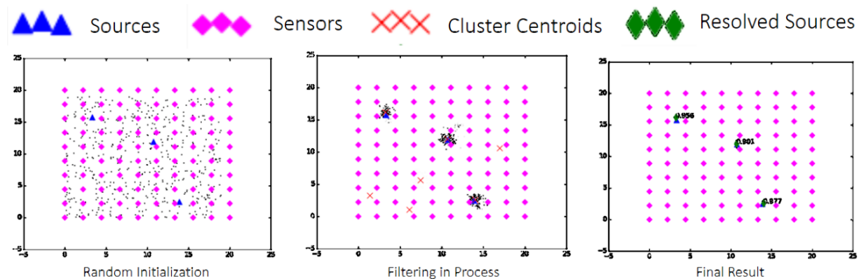
Figure 2.7: Locating sources using a particle filter 6
