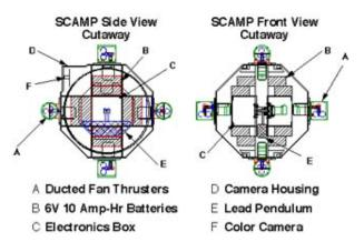
Figure 4: Cutaway view of the Supplemental Camera and Maneuvering Platform
