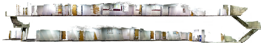
Figure 7.3: Dense mapping system based on planar surfaces [99]. The factor graph is similar to structure from motion, but with infinite planes instead of point features.
