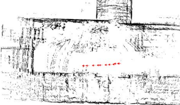
Figure 7.11: IRLS-ICP, Trimmed ICP, MDME (our proposed method) : This is a top-down view of twelve frames of LIDAR data that were registered frame-to-frame and then plotted in a global coordinate system. The ground points have been removed for clarity. Look to the northern corridor for the clearest signs of registration error. Note the severe inadequacy of Trimmed ICP, which produces too little movement. Our proposed method without EOE does fairly well, but performs best with the addition of EOE.
