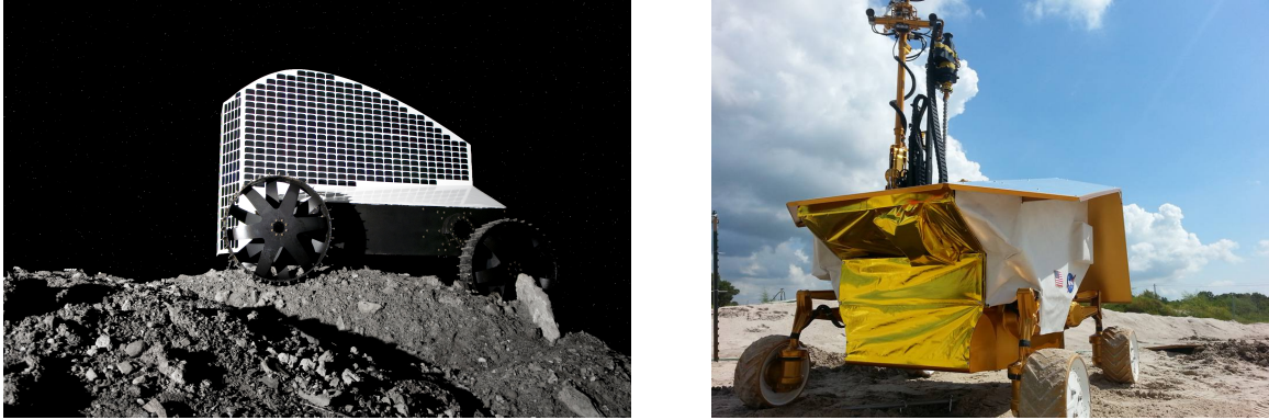
Figure 1.1: Prototype solar-powered lunar polar rovers. Left: “Polaris” (Image credit: Astrobotic Technology, Inc.) Right: “Resource Prospector” (Image credit: NASA)
