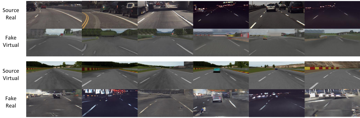
Figure 4.5: Image generation results of CycleGAN. Top row: real source images and generated fake virtual images. Bottom row: virtual source images and generated fake real images.
