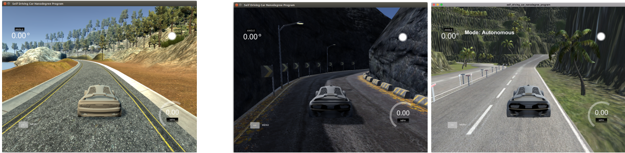
Figure 3.3: Sample screenshots of the environment in the Udacity autonomous driving simulator. The left one shows the training track in the desert, while the two on the right show the test track in suburb and mountain. The test sets are different from the training set regarding lighting conditions, curvature, inclination, road geometry and off-road scenery and thus are considered much more difficult.
