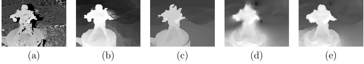
Figure 4.3: Inverse depth map comparison (a) MVP M (b) Ha et al. [9] (c) MVP M+Yang [19] (d) Naive depth reconstruction without occlusion and gradient weights (e) MVP M + Deep Normals
