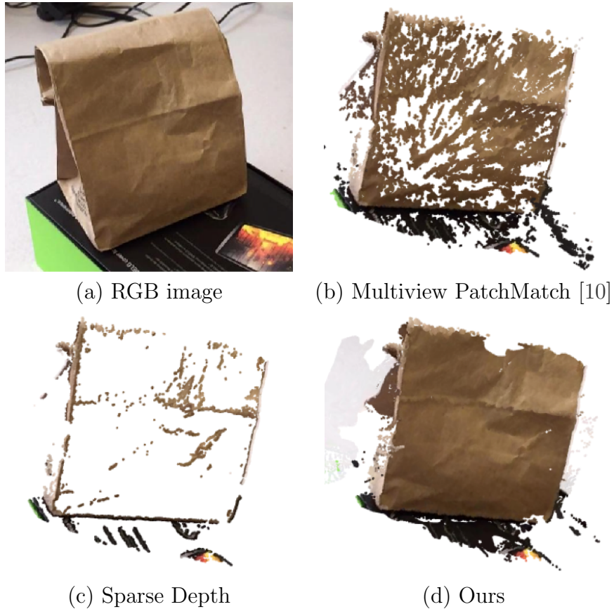
Figure 4.1: Depth reconstruction from small-motion videos. Traditional methods give noisy depth estimation in low-texture regions as (b). We use surface normal prediction to fill the holes in sparse depth map in (c) and improve depth estimation accuracy in low-texture region as shown in (d)
