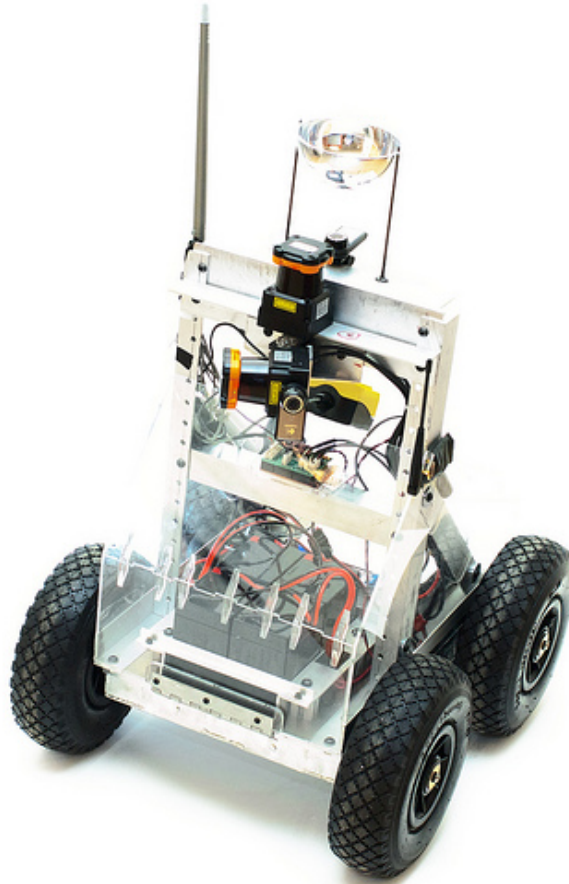
Figure 5.5: One of the University of Pennsylvania’s MAGIC2010 robots. The robots used two laser range scanners, an omni-directional camera, and a panning camera to gather information about the environment. An on-board Mac Mini provided computational power, and a 802.11 antenna provided the data link with the ground control station (GCS). (Photo © 2010 Paul Vernaza)
