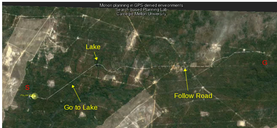
Figure 6.11: An example route showing GOTO LAKE, METRIC MOTION, and FOLLOW ROAD controllers while operating in GPS-denied environment.
