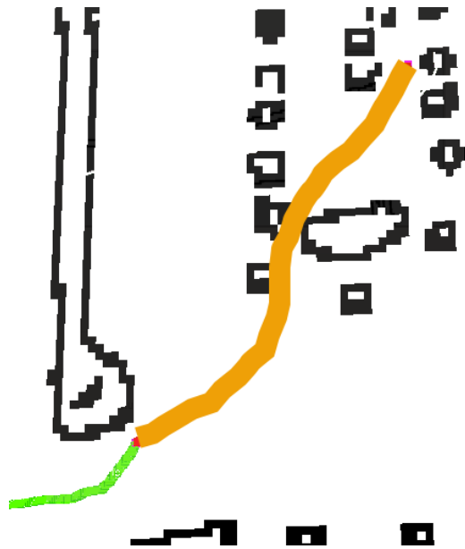
Figure 6.16: An example of the EXECUTEMOTIONPRIMITIVE controller moving down to the left. The thick sections in the center do not have an adequate wall or landmark near by, so the planner uses several of the standard motion primitives to avoid the obstacles. Note: the line is drawn thicker than the robot footprint for clarity; the robot trajectory remains collision free.
