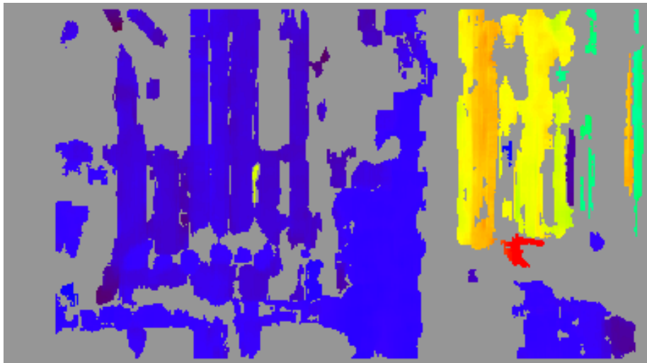
(b) Disparity image generated from image pair. Red is largest disparity (closer) and purple is smallest (farther).
