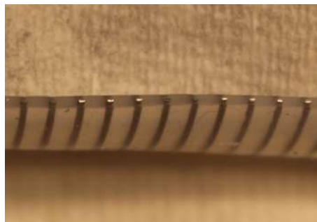
FIGURE 4.9: Cross-section of the Sensor. The resulting cross-section shape of the eGaIn pattern is approximately semicircular.
