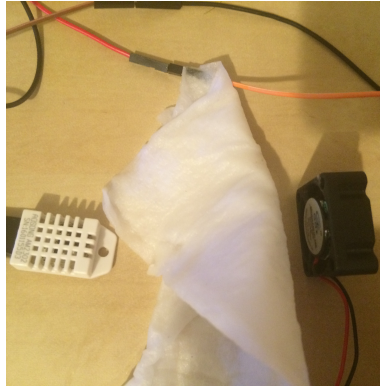
Figure 14: Tissue with water and 5v mini fan was used to decrease humidity
