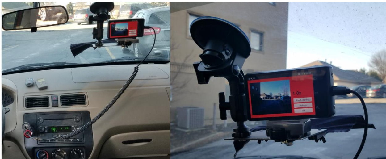
Figure 2: Data collection setup: A smart phone is mounted on the windshield with a setup similar to a GPS mount. The collection app is running on the phone.
