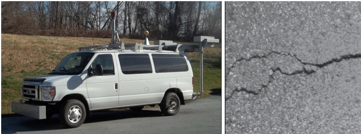
Figure 1: Left: Mobile Data Recorder (MDR) used by the Pennsylvania department of transportation for automatic pavement distress condition surveying. Right: High resolution images of the road taken by specialized downward facing cameras.
