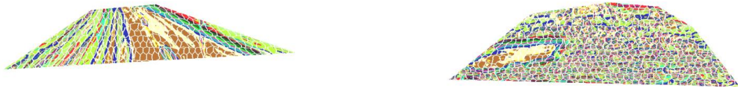
Figure 5: Texton maps generated of the example images shown in Figure 4. Notice that the textons are generated only on the masked area
