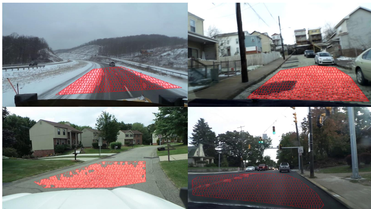
Figure 7: Sample results of testing phase. Coloured ones denoting the predictions made by the SVM classifier. Classification result for snow covered road (left-top). Areas where the road is clear is shown to be negative. Results for cobblestone-vs-asphalt road area (right-top), cracked road (left-bottom) and good road (right-bottom).
