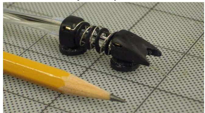
Fig. 9. HeartLander. Suction is applied to each of the two round feet in order to adhere to the epicardium. The device crawls like an inchworm, using wires to advance the front foot and then sheaths surrounding the wires to push the rear foot up to meet the front. Steering is performed by advancing unequal lengths of the three wires. The device includes a videoscope for visual feedback, and is controlled via joystick by the surgeon. Numerous end-effectors are possible; the prototype shown incorporates a retractable needle for injections (shown partially extended for visibility).
