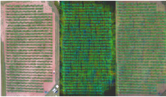
Fig. 7. (Left) An aerial view of sorghum test plots in Clemson, SC. (Center) Laser scan data of the same test plots corrected using calculated vehicle pose estimate. (Right) Overlay of two images, indicating accuracy of pose estimation.
