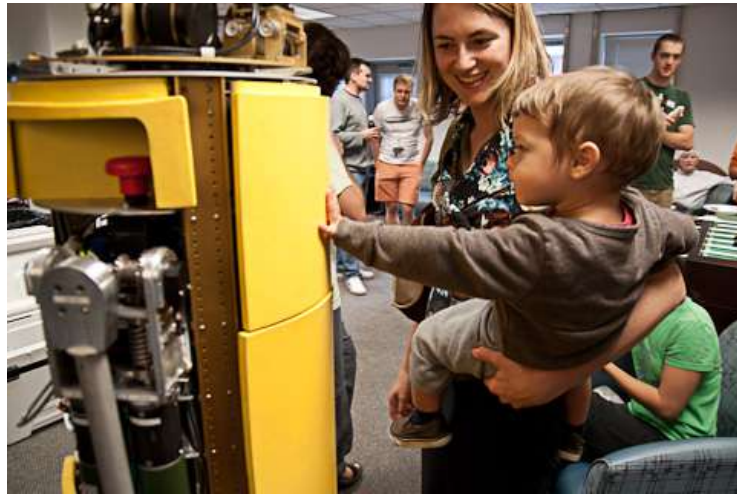
(b) A demonstration of the ballbot's physical compliance. A small child is pushing the 65 kg robot, and it moves away.
