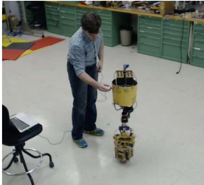
Figure 6.22: Testing force estimation with a force gauge.
