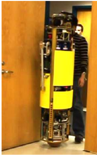
(a) The ballbot navigating through a doorway. This maneuver is made easier because the robot has a relatively small footprint for its size.
