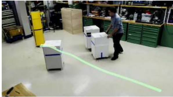
(a) The ballbot initially starting at rest at t_0 = 0 s. A straight path to the goal in the lower right is planned.
