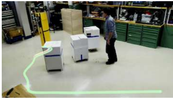
(c) At t_1 = 4 s, a box is placed blocking the straight line path, and the ballbot replans smoothly to go around the obstacles.
