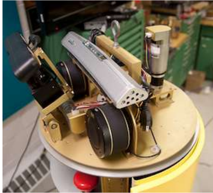
(b) The ballbot's pan/tilt turret with microphone, speakers, point cloud sensor, and laser scanner
