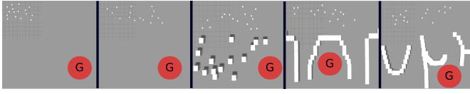
Fig. 2: The 5 maps in Gazebo used for our experiments. Maps From left to right 1 (Empty Map Dense with spawn region ([1-6], [1-8])), 2 (Empty Map Spread with spawn region ([1-6], [1-19])), 3 (Uniform Map), 4 (Corridor Map), 5 (Concave Map). The goal region is the red disk labeled G, with robots (White) spawning in the upper region. Robots spawn in the x in [1,6], y in [1,19] range for all maps except empty dense.
