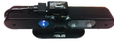
Fig. 2: The IMU (Microstrain 3DM-GX4-25) is rigidly attached on the top of the RGB-D sensor (ASUS Xtion Pro Live).
