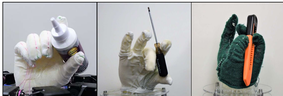
Figure 4.7: Demonstration of static grasping with a glue bottle (left), a screwdriver (middle) and a box cutter (right).
