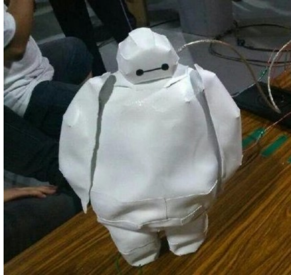
Figure 4.12: An inflatable robot built using solder iron for sealing the plastic cloth.
