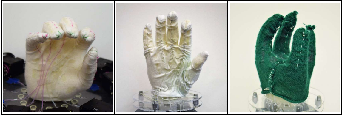
Figure 4.4: Rest poses of three foam robots. From left to right: 1) Anthropomorphic hand in a cupping pose; 2) Anthropomorphic hand in extended pose; 3) Non-anthropomorphic hand in caging grasp pose.
