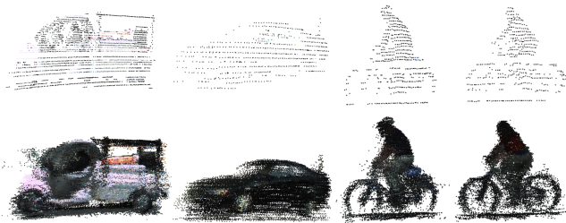
Fig. 8. Models obtained by tracking objects. The top row is the individual frame of the tracked object with the highest number of points. The bottom row is the model created by our tracker. Note that we are only performing frame-to-frame alignment when building these models.
