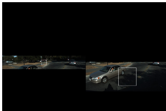
Fig. 4. Left: We black out the image except near the horizon, to search for smaller cars. Right: We black out the image except lower pixels, to search for larger cars. The white boxes indicate the scale of car that is being searched for in the image. By limiting our search space at each scale, we get better performance and a large increase in the speed of our algorithm.
