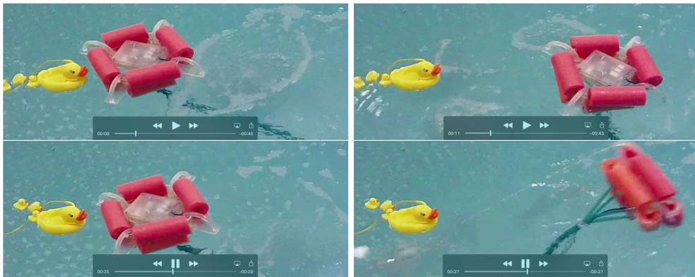
Figure 4.4: Storyboard of shy behavior movement through time steps. *Firefly* slowly approaches the interaction object (rubber ducks) from multiple angles. The robot always keeps distance between the ducks and never physically bumps the ducks. Additionally, *Firefly* will rapidly hops or moves away from the ducks after some amount of time approaching them.
