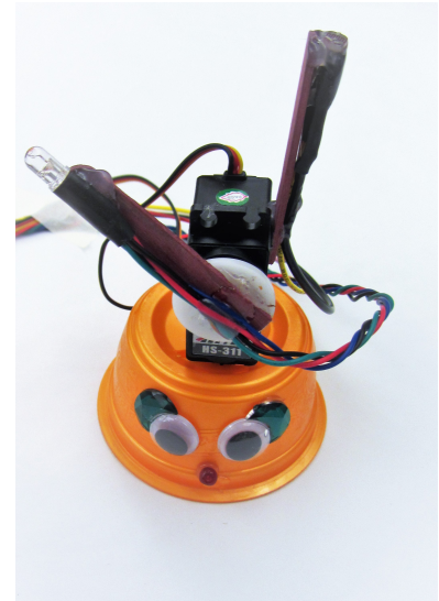
Figure 4.1: Example mini-bot robot with a servo light sensor and tri-color LED..
