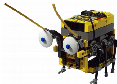
Figure 2.1: A insect-like, walking robot built with LEGO MINDSTORMS by Mario Ferrari. ( www.marioferrari.org/lego/brlm/brlm.html )
